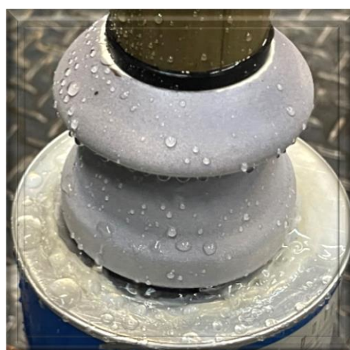
Fig. 4. The effect of silica loading of the coating suspension on WCA
