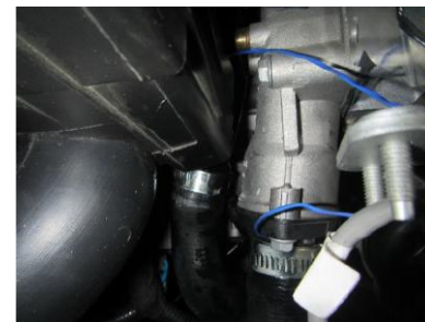
Figure 5: The inlet and outlet water temperature sensors of radiator on the vehicle
