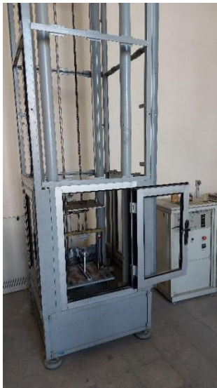
Figure 8: DCB impact test setup.
