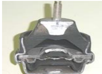
Fig24. Hydraulic engine mount with Inertia track
