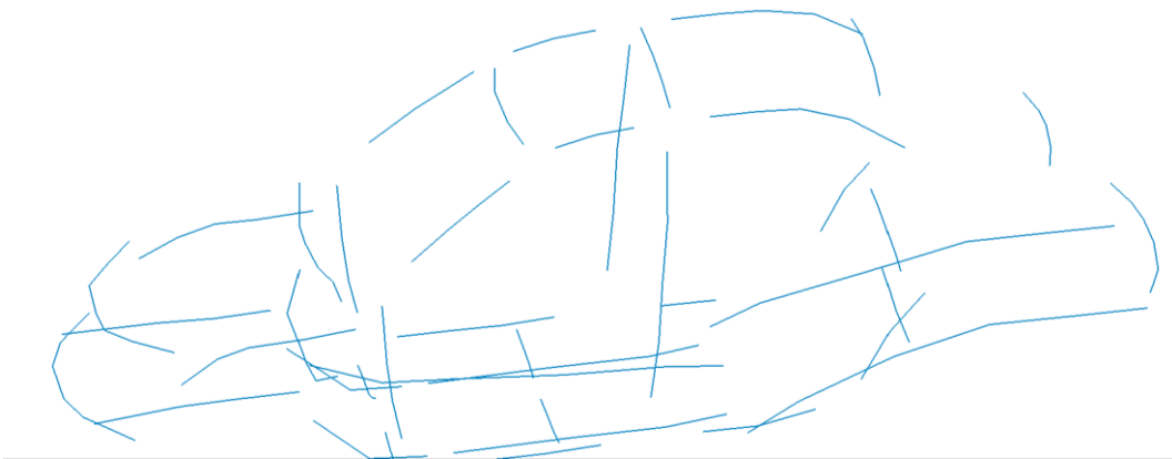
Fig3.: Equivalent beam modeling of the BIW
