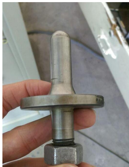
Fig2. Steel imp actor used in drop ball tests
